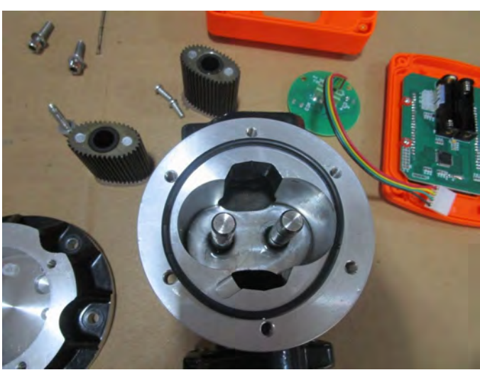
Product internal inspection
